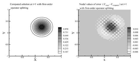
Fig. 6. Horizontal slice (on z = 0 plane) of the computed scalar field (left panel) and the error field (right panel) after 10 time steps of 0.1 in a  $30 \times 30 \times 30$  grid with first-order operator splitting approach (test case 2: advection–diffusion of a Gaussian sphere).
