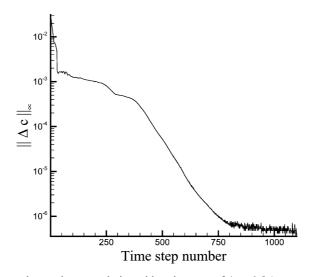
Fig. 12. Convergence history to the steady state solution with a time step of  $\Delta t = 0.5$  (test case 3: Graetz–Nusselt solution).
