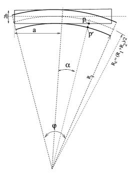
Fig. 10. A schematic of the mapping used to create the mesh in test case 3 (Graetz–Nusselt problem). Solid lines represent the box in which the structured mesh was generated. Heavy lines represent the 15-degree annulus sector used as the computational domain.
