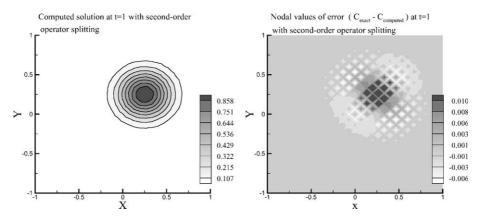
Fig. 7. Horizontal slice (on z = 0 plane) of the computed scalar field (left panel) and the error field (right panel) after 10 time steps of 0.1 in a  $30 \times 30 \times 30$  grid with second-order operator splitting approach (test case 2: advection–diffusion of a Gaussian sphere).
