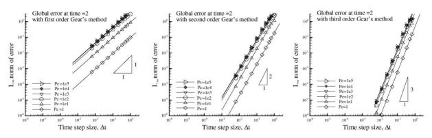
Fig. 2. Global error at time t = 2 versus  $\Delta t$  with (from left to right) first-, second- and third-order Gear's backward time stepping methods. The slope of error plots in log–log scale is indicative of the order of the scheme (test case: algebraic solution testing for diffusion).
