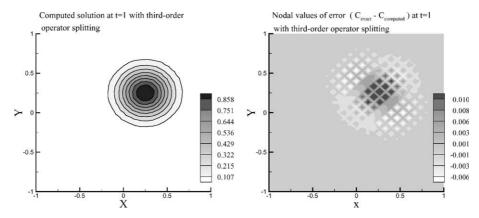
Fig. 8. Horizontal slice (on z = 0 plane) of the computed scalar field (left panel) and the error field (right panel) after 10 time steps of 0.1 in a  $30 \times 30 \times 30$  grid with third-order operator splitting approach (test case 2: advection–diffusion of a Gaussian sphere).
