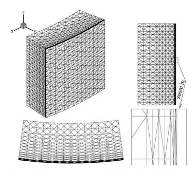
Fig. 11. A close-up of the mesh used for the test case 3 (Graetz–Nusselt problem). A 3-D view is shown at top left, a z = constant slice is shown at bottom, and a x = constant slice is shown at right.
