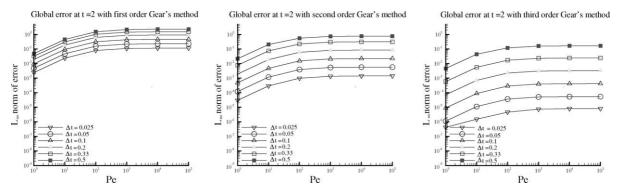
Fig. 3. Global error at time t = 2 versus *Pe* obtained with various time step sizes. The three panels represent results using (from left to right) first- through third-order Gear's backward differencing scheme (test case: algebraic solution testing for diffusion).
