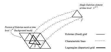
Fig. 1. Schematic of Eulerian and Lagrangian grids for a characteristic Galerkin method.
