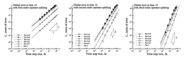
Fig. 5. Global error at time t = 2 versus  $\Delta t$  with (from left to right) first-, second- and third-order operator splitting methods (test case 1: algebraic solution testing for advection–diffusion).
