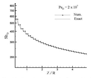
Fig. 13. Dimensionless gradient of the solution (Sherwood number  $Sh_D$ ) on the wall versus axial position (Z/R) for test case 3: Graetz–Nusselt problem.
