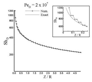
Fig. 14. Dimensionless gradient of the solution (Sherwood number  $Sh_D$ ) on the wall versus axial position (Z/R) for test case 3: Graetz–Nusselt problem with the refined mesh. Comparison with Fig. 13 reveals that the step pattern is suppressed to a great extent as the mesh is refined. The inset shows a closer look at the inlet region, where the near zero boundary layer thickness prevents full capture of the solution gradient.
